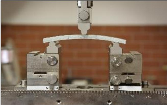
Figure 1: Three point bending test (ASTM D 790)
