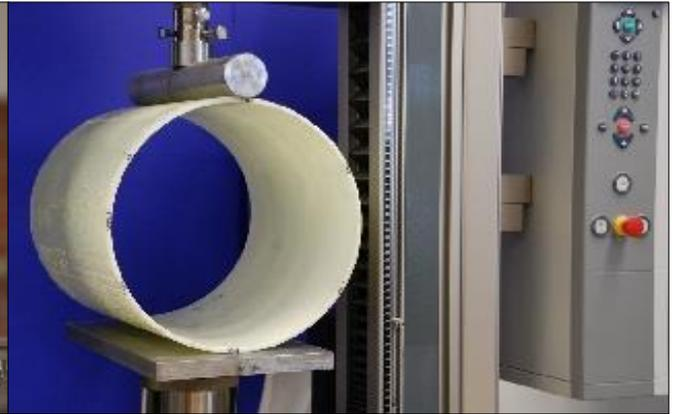
Figure 2: Parallel plate test (ISO 9969)
