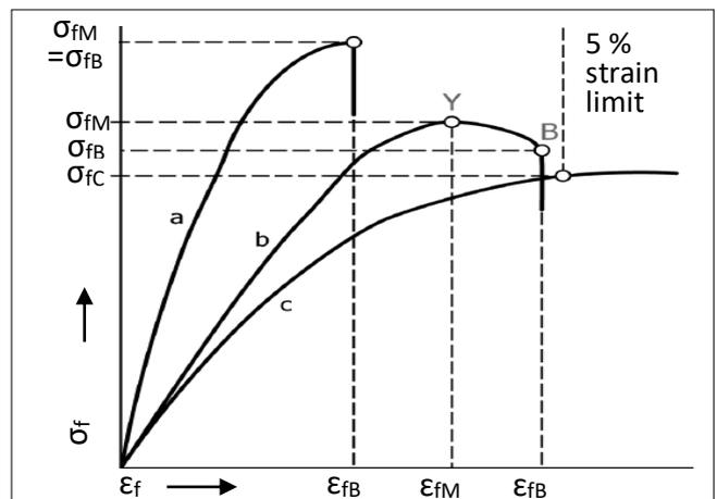
Figure 7: Flexural Stress ( $\sigma_f$ ) Versus Flexural Strain ( $\epsilon_f$ )
