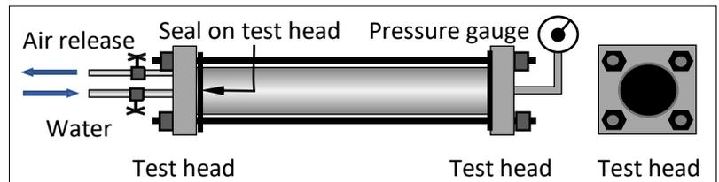
Figure 3: Hydrostatic pipe test between test heads
