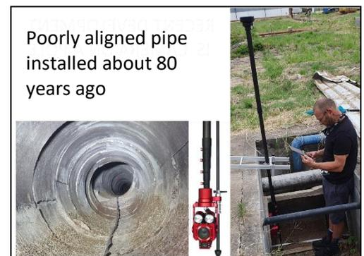
Figure 1: Camera on pole inspection
