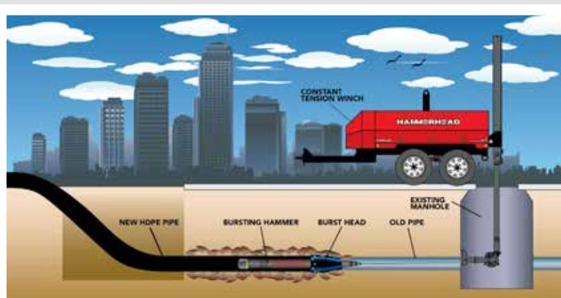
“One of the ideal approaches for the replacement of large-scale pipes is the application of pipe-bursting technology, an area where Gokor Construction has expert experience. At the business end is a purpose-built Hammerhead HG12 and Hydroguide pipe-bursting system, supplied and supported by local distributor ELB Equipment.
